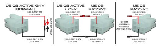
To connect the US OB PASSIVE to the ACTIVE, connect the 2 Asia plug connections with one another (see figure). You can also operate the US OB PASSIVE on another power amplifier by using the SUB inputs.
