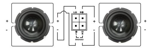
voice coils are wired in parallel and wired to each channel for a 2 Ohm load on each channel
