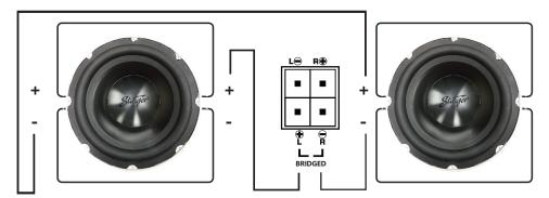
All voice coils are wired in parallel, then each speaker in series for a 8 ohm bridged load
